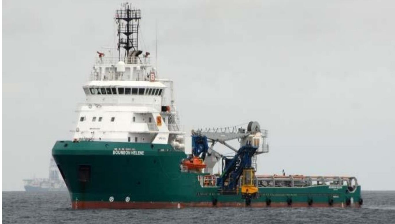
BOURBON HELENE is a GPA 670 design, diesel electric, DP 2, multipurpose subsea services support vessel with one AHC deep water crane and accommodation for 44 persons.
